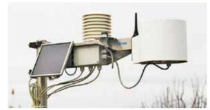
The Weather Stations, powered by a solar panel, transmit weather data in real time over GSM/GPRS.
