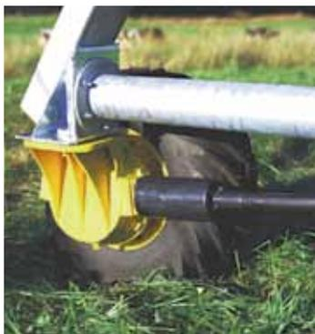
*Growers, particularly those producing turf, forage and vegetables, will benefit from the AcreMaster's high flotation ag tires. With low ground pressure, they reduce tire rutting problems.*
