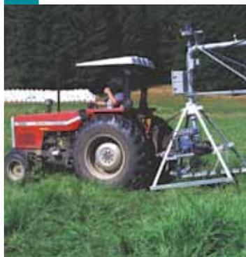
*The three-point hitch configuration and low profile pivot point make the lightweight AcreMaster easy to tow and reposition. Once in place, it may be secured with earth anchors, eliminating the need for concrete pads.*
